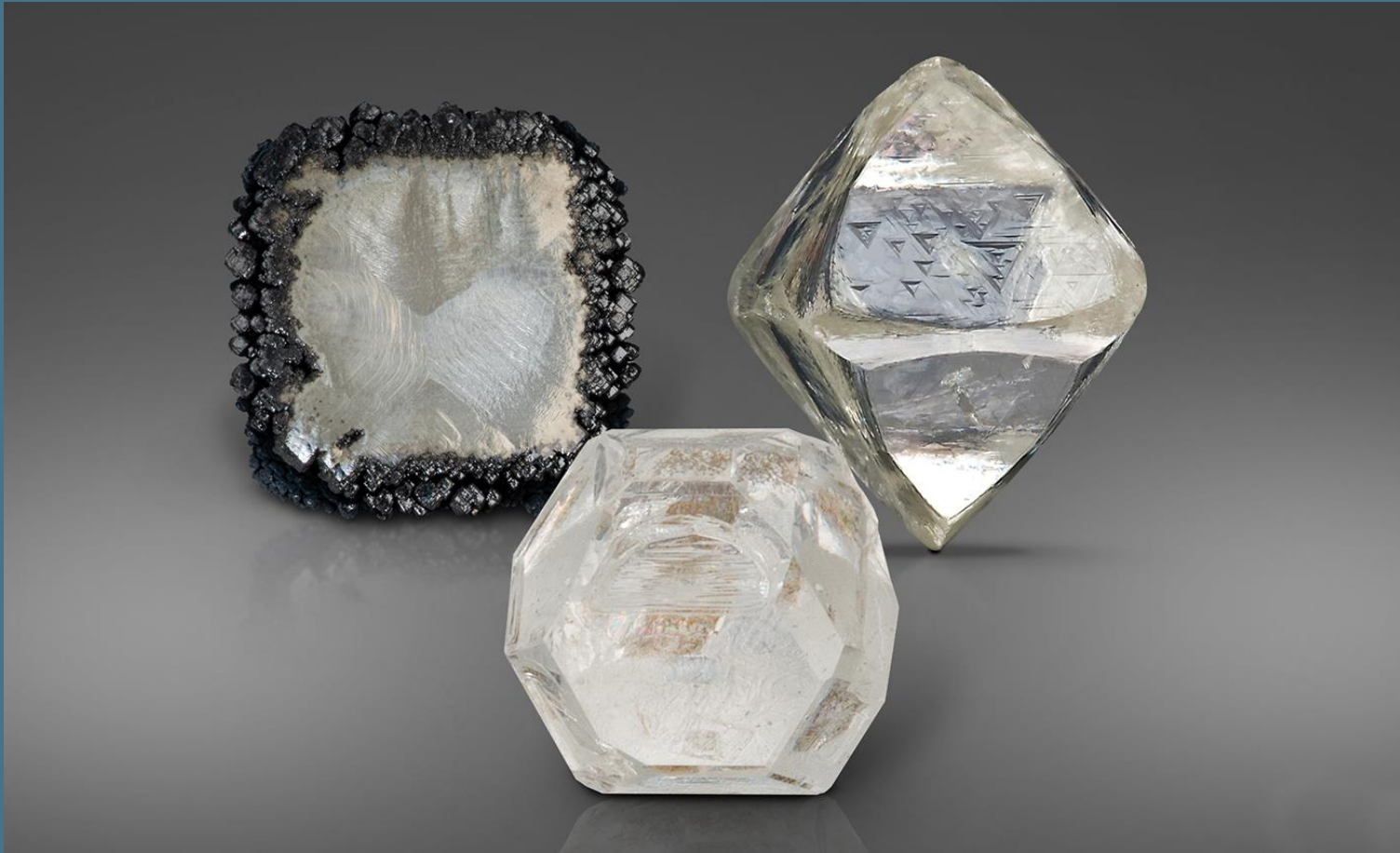
From left to right: lab-grown CVD rough diamond, lab-grown HPHT rough diamond, and natural rough diamond
